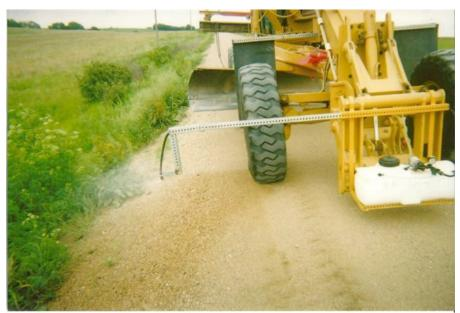
adjustable with the side bar on sprayer and up or down with the motor grader front bar assembly. The sprayer is controlled by a toggle switch inside the cab. Various chemicals such as brush control can be applied as needed.
