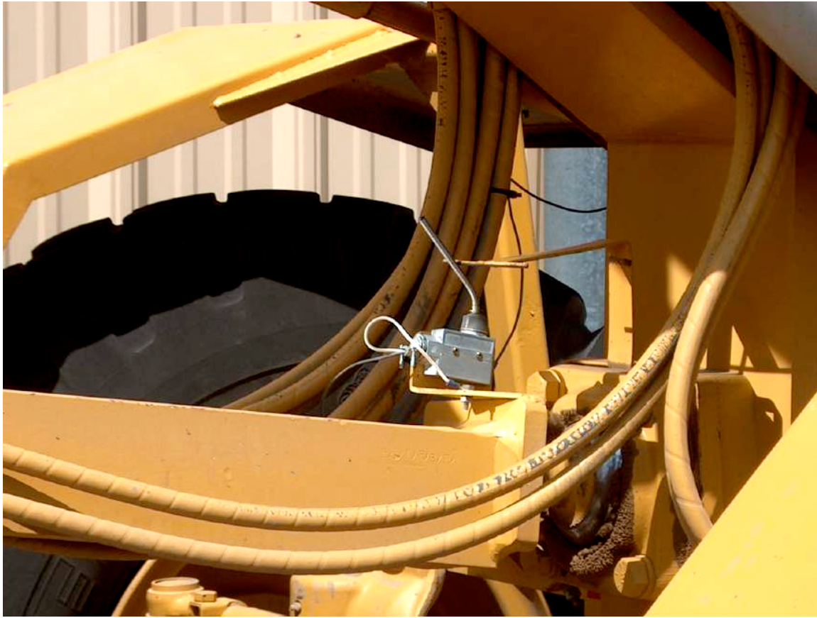
View #4 Micro-switch that automatically raises and lowers the magnet as the operator raises and lowers the blade.
