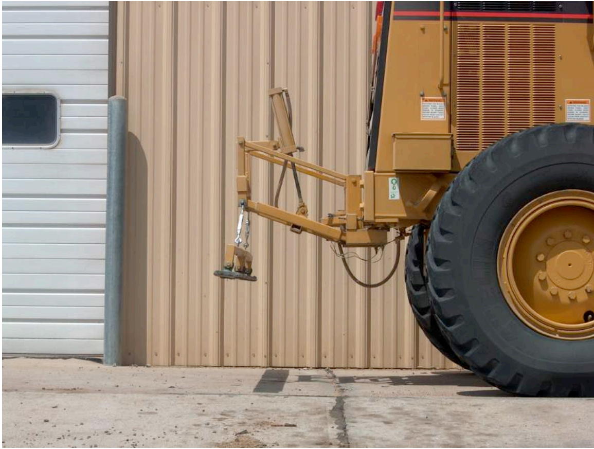
View #2 Magnet shown in up position.
