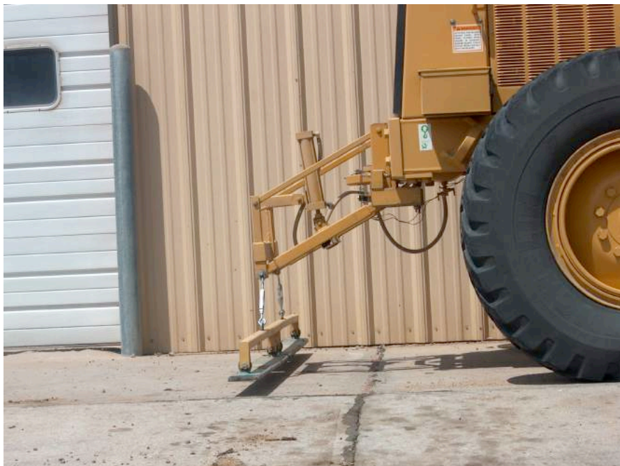
View #1 Shows Magnet in down position.
