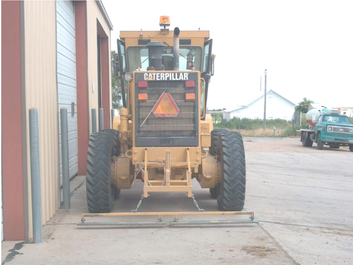
View #3 Magnet shown from behind, in down position.
